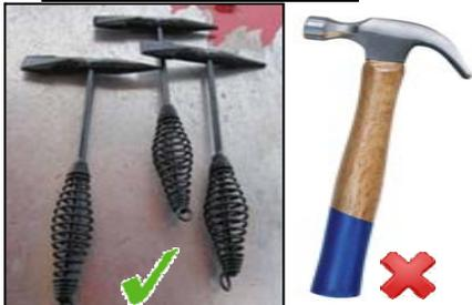
On the 19th April 2013, a LCQ mechanic sustained a 1cm laceration of left index finger due to the hammer head of the wooden hammer being loose, hence causing the finger injury. The lesson learnt from this injury is to phase out the wooden hammers and replace it with certified metal or silicon hammers.
